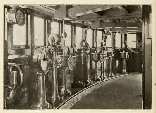
BRIDGE OF THE "LUSITANIA" Showing the Engine Telegraph, Telephones, Signals, etc.
