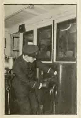
Closing the Bulkhead Doors in Twenty Seconds from the Bridge
